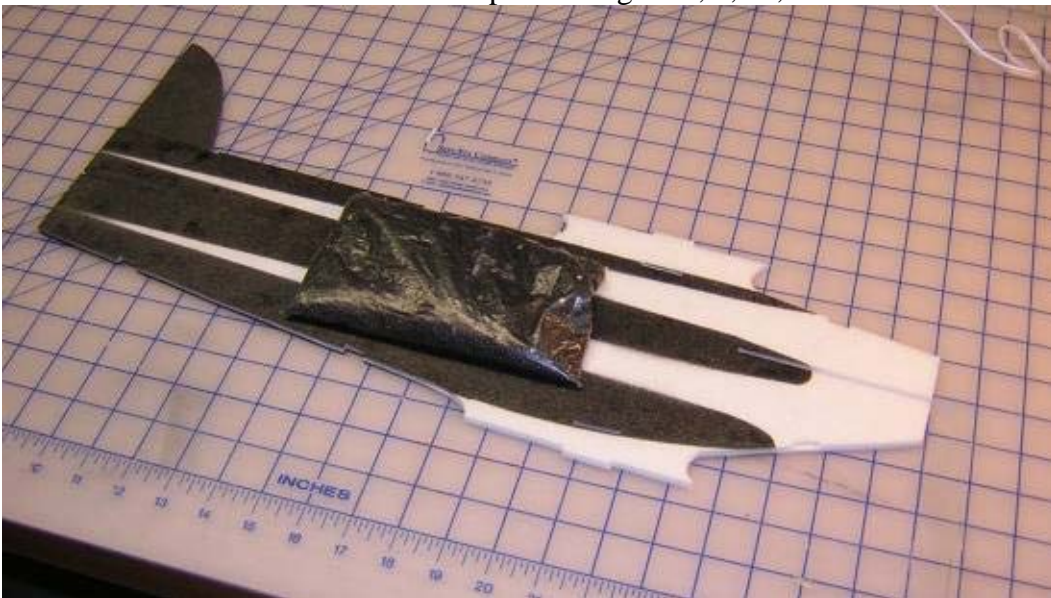
Figure 6: Stack fuse halves keeping perfectly aligned.
