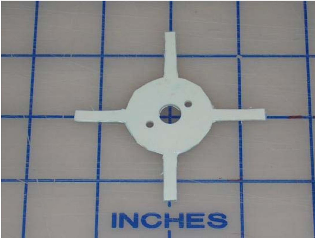
Figure 15: Motor mount cut from ABS plastic.
