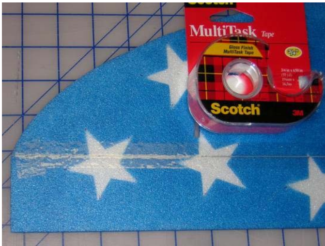
Figure 11: Tape on ailerons and elevators with \frac{3}{4} " clear tape.
