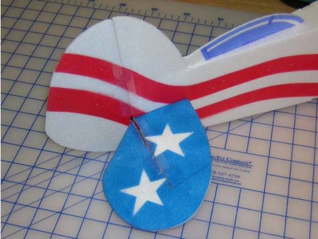
Figure 14: Glue in tail feathers ensuring they are perpendicular to fuse.
