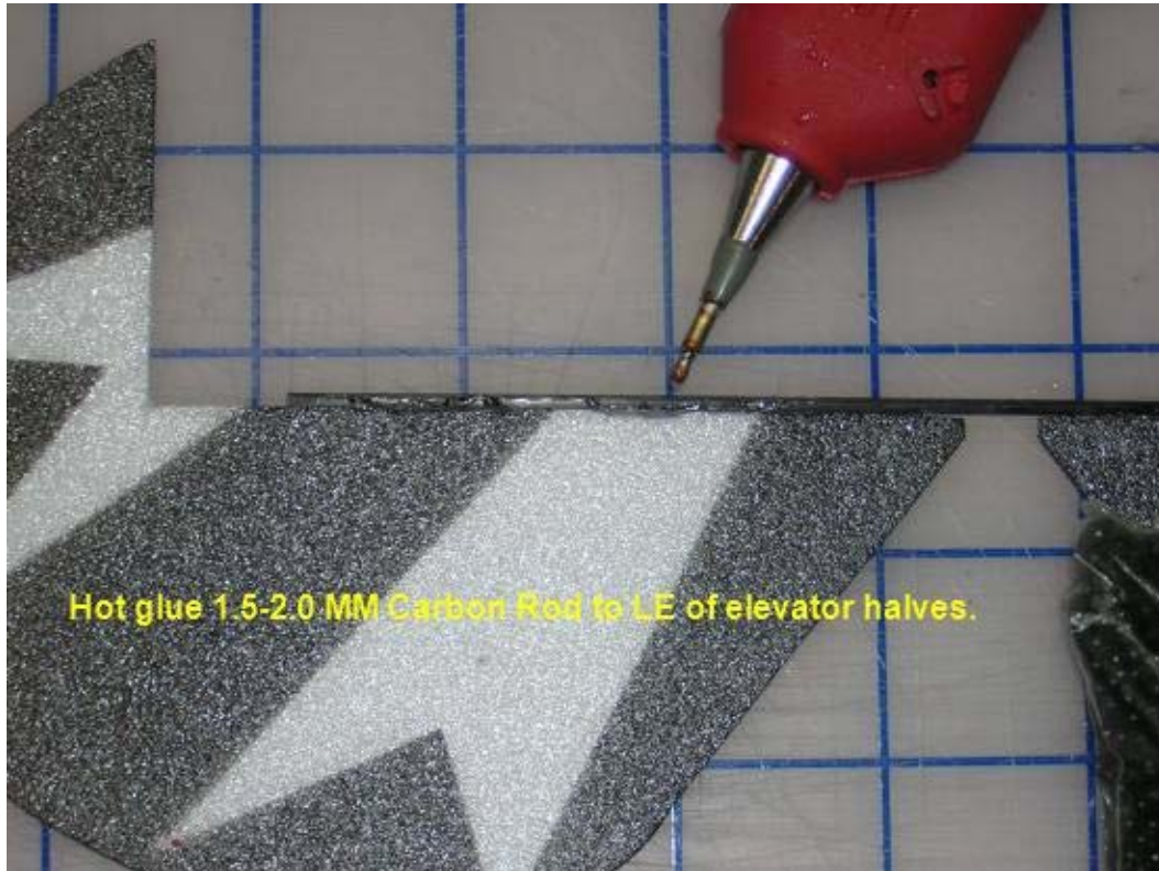
Figure 10: Hot glue elevator halves to carbon fiber rod.
