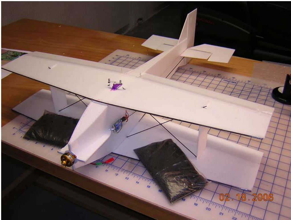
Figure 16: X-bracing the wing. This is the Perfexion, but it is the same on the Football. Note how carbon rod was “poked-in” from above and then cut to length after glue sets. Repeat process for other braces. The braces are for rigidity and drag. Yes, drag is good on indoor models!
