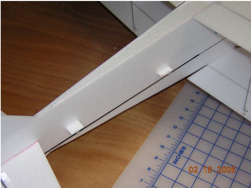
Figure 21: RX is taped to fuse side along thrust line. Again, Perfexion model shown here, sorry, that is the photo that I have. Eventually I'll tuck the RX inside. Note how everything is along thrust line!
