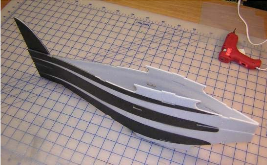
Figure 8: No, it is not Shamu the killer whale, it is the fuselage ready for top and bottom formers! Note how rear of fuse is flat until front of fin. Note that the final plans have only two slots for fuse formers – I eliminated the additional tabs shown on these photos.
