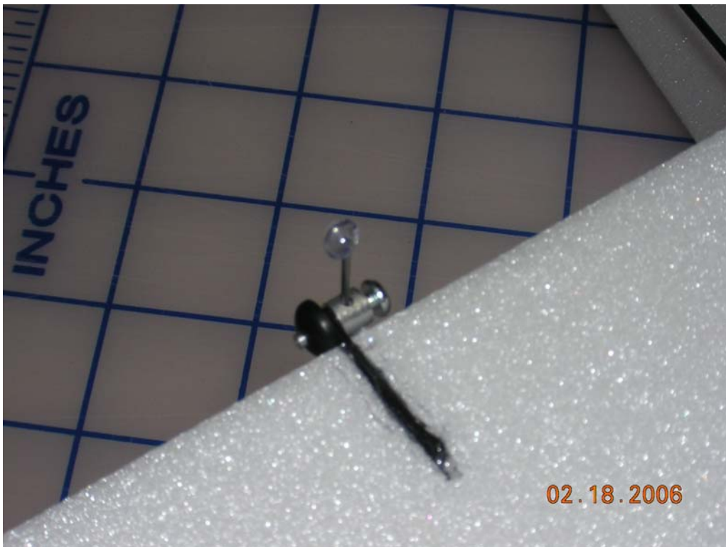
Figure 17a: I use cut-off zip tie ends for the aileron linkages. Drill hole through end and insert Dubro micro hardware. Connect the two ailerons with 1.0 mm carbon rod or wire.
