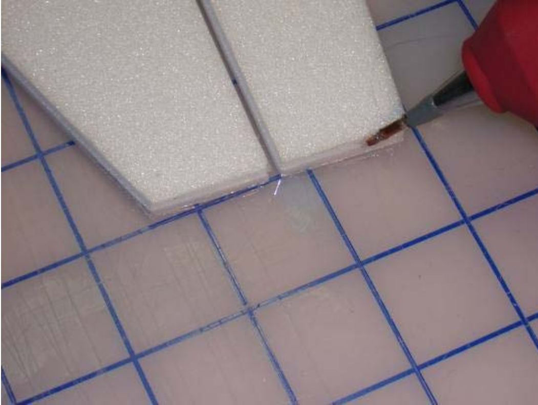
Figure 7: Hot glue both ends of fuselage to form an envelope. I run a bead and then “smear” it flat to form a flexible bond.
