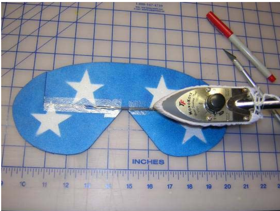
Figure 12: Iron on tape with iron set at #1, warm.
