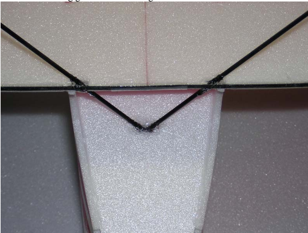
Figure 19: Hot glue landing gear in place as shown. For real strength you can wrap the
