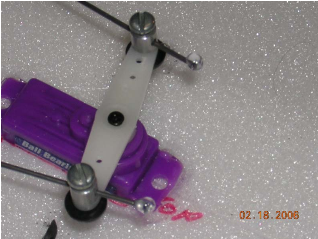
Figure 17: Aileron servo glued in to top of wing. Dubro micro hardware is used at both ends. Pushrods for ailerons are just 0.040 music wire.
